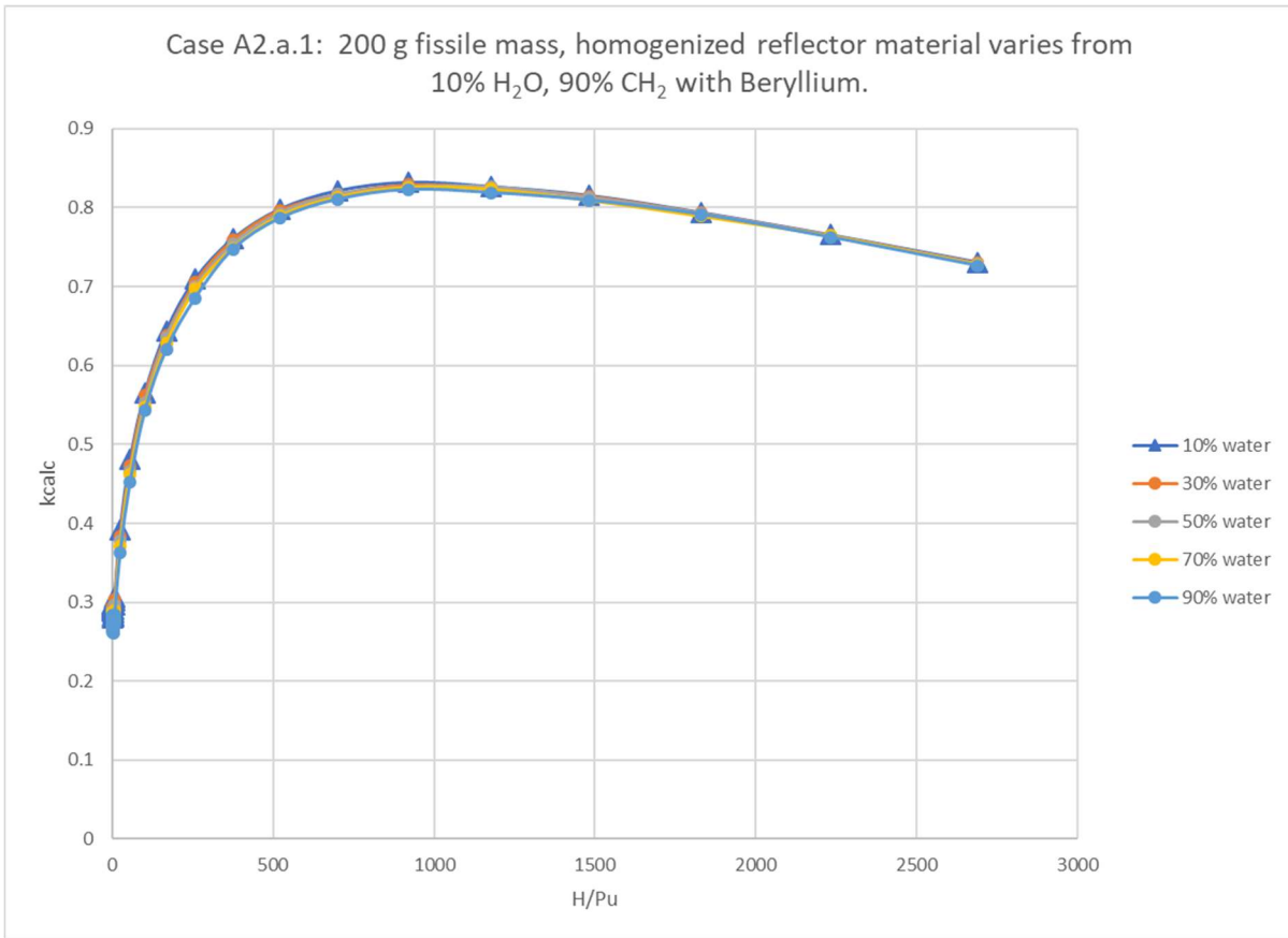
Figure A-5. H/Pu study, waste form is 200 g 239 PuO 2 , 75% H 2 O with 25% CH 2 ; reflector is homogenized beryllium with 10–90% H 2 O and 90–10% CH 2 ; infinite salt reflection.
