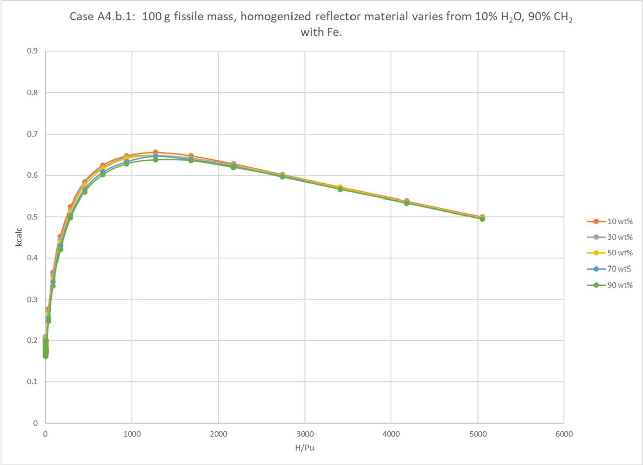
Figure A-14. H/Pu study, waste form is 100 g 239 PuO 2 , 75% H 2 O with 25% CH 2 ; reflector is homogenized 10–90% H 2 O and 90–10% CH 2 with 0% beryllium and Fe; infinite salt reflection.
